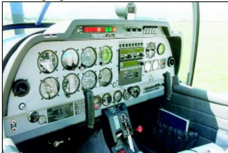
Simple effective cockpit with dual throttles and no plastic trim save the centre console.
