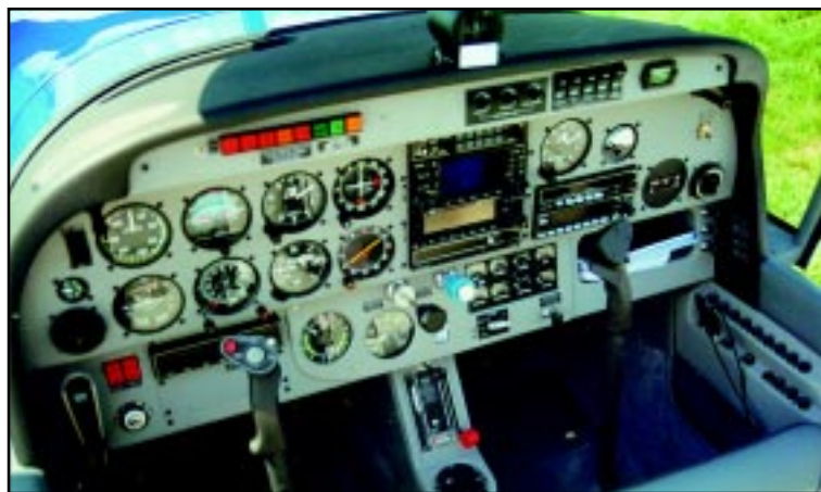
ZK-TZA has very comprehensive instrument fit including dual GPS receivers.
