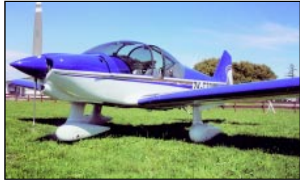
Smoothed off cowlings and wheel pants are features along with the sharp spinner. Superb all round visibility is a feature not only for aerobatics but when in the circuit.
